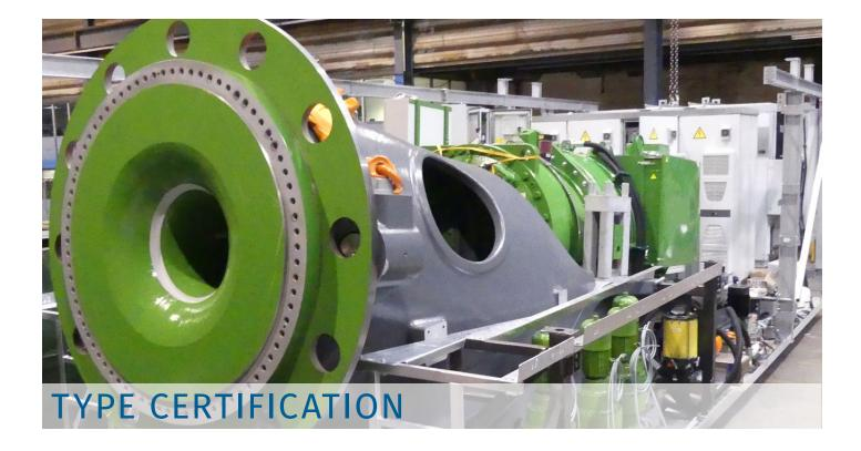
Type certification attests that your wind turbine or its components comply with all applicable directives and standards. This includes the examination of the design documentation and the evaluation of the manufacturing and the prototype test.
