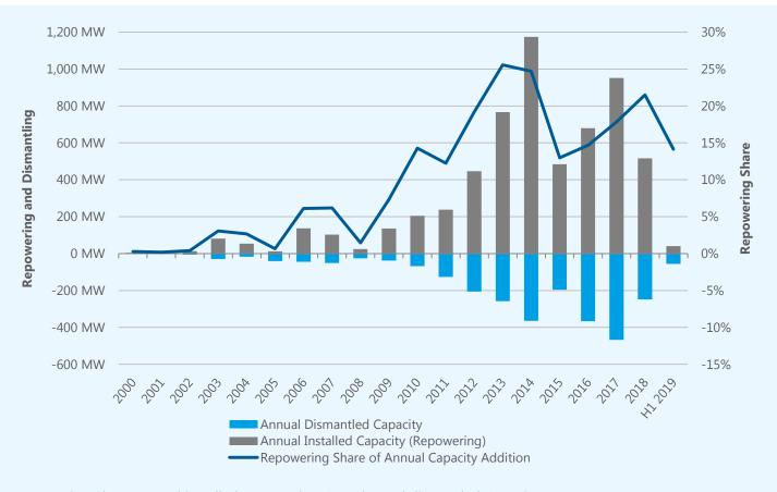
Repowering Share, annual installed Repowering Capacity and dismantled Capacity
