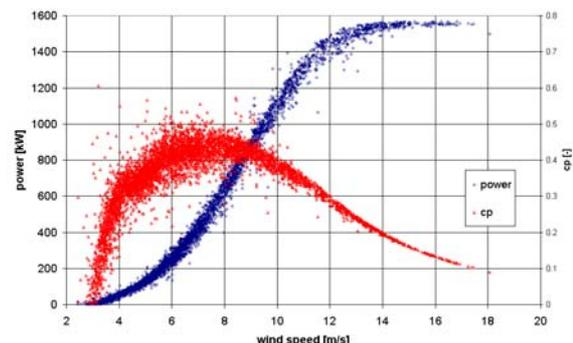
Fig. 5: Raw data plot of power curve and power coefficient
