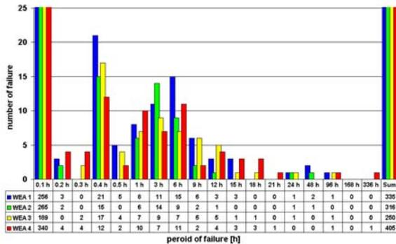
Fig. 8: The Analysis of the duration of downtimes shows how long the turbine, the technical wind farm operator and the service team of the manufacturer need to eliminate the errors.
