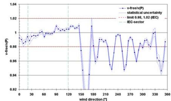
Fig. 4: Self-consistency test for assessing the wind direction sector for power curve evaluations.
