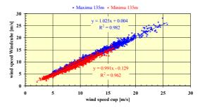
Figure 12: Comparison of extreme values of wind speed within 10-minute periods as measured by Windcube and a cup anemometer at 135 m height (4 second cone rotational mode).
