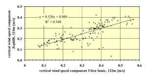
Figure 7: Comparison of vertical wind speed component measured at 124 m height above ground by ZephIR and measured at 122 m height above ground by an ultra sonic anemometer (10-minute averages).
