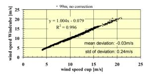
Figure 2: Comparison of 10-minute averages of horizontal wind speed component measured with the Windcube prototype and with a cup anemometer at 99 m height.
