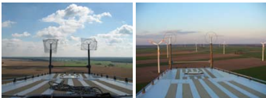
Figure 3: Different arrangements of anemometers/vanes on nacelles observed in the same wind farm leading to massive production losses covered neither by exemplary
