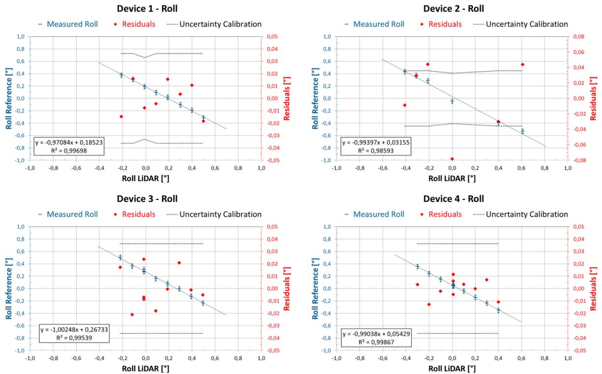
Figure 5: Calibration results of the roll angle of the LiDAR. Blue markers are the reference roll as function of the roll given by the LiDAR. The error bars denote the standard uncertainty. The red diamonds give the residuals, i.e. the deviation between the shown calibration line and the measured values. The dotted lines denote the standard uncertainty of the calibration on the axis of the residuals ( $k=2$ ).
