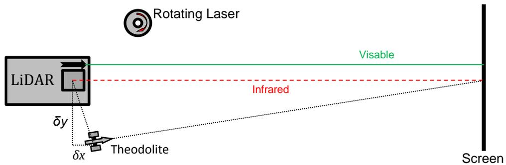
Figure 2: Top view of measurement setup. The rotating laser transfers the reference height  $h_0$  from the LiDAR to the theodolite (Method A) and the screen (Method B). The longitudinal and transversal displacements of the theodolite,  $\delta x$  and  $\delta y$ , are components of the uncertainty budget of Method A.
