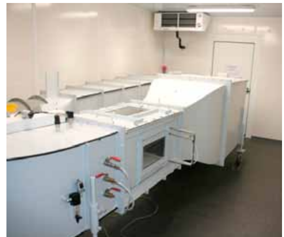
Figure 2: Photo of the Variable Air Density Wind Tunnel of Windguard Wind Tunnel Services
